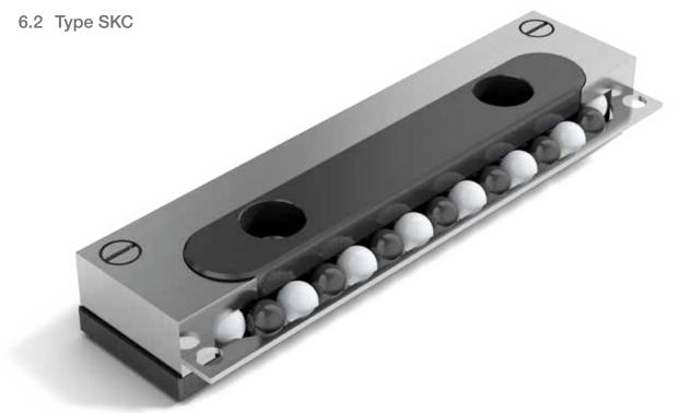
The recirculating unit type SKC was developed for dry runs and in-vacuum and clean-room applications. It is made out of DURALLOY® coated steel and has ceramic balls, which are separated from one another by balls made out of TEFLON®.
